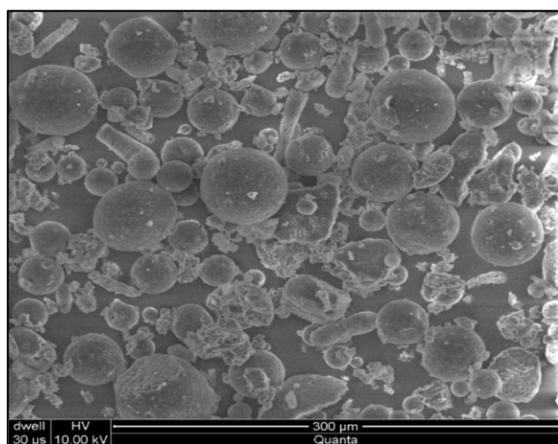
**Fig. 7: Scanning electron microscope image of Vitamin D<sub>3</sub> microsponges prepared by O/W (F<sub>8</sub>)**
