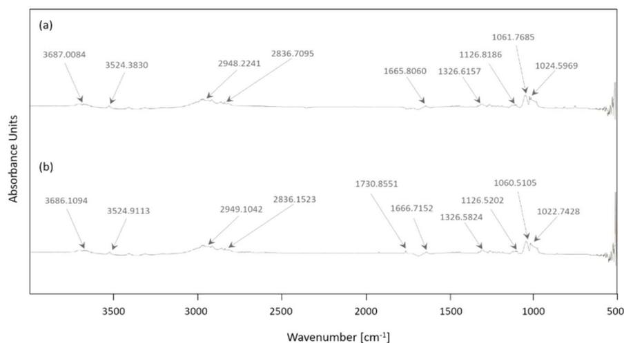
Fig. 4: FTIR spectra of (a) pure and (b) encapsulated ascorbic acid
