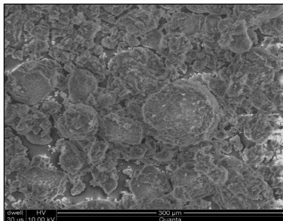
**Fig. 6: Scanning electron microscope image of Vitamin C microsponges prepared by W/O/W (F<sub>5</sub>)**
