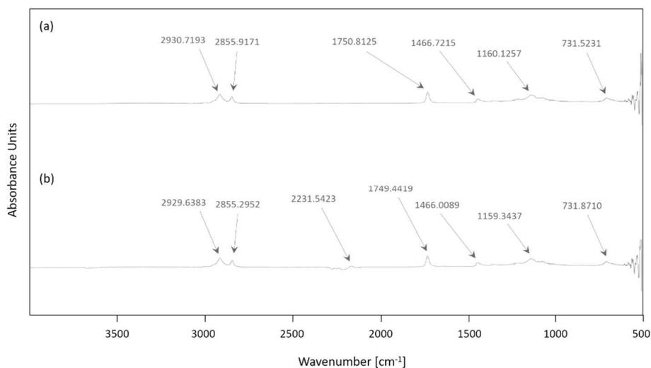
Fig. 5: FTIR spectra of (a) pure and (b) encapsulated cholecalciferol
