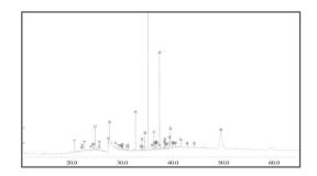
Fig. 4: Gas chromatogram of the ethyl acetate extract of the leaves of *N. cadamba*. Benzaldehyde (1), benzyl alcohol (2), pentanoic acid, 4-oxo-, phenylmethyl ester(6), benzyl ether (8), tetradecanoic acid (10), n-hexadecanoic acid (16),octadecanoic acid, ethyl ester (21), 1,2-benzenedicarboxylic acid, diisooctyl ester (28), progesterone (42), and tetratetracontane (45)
