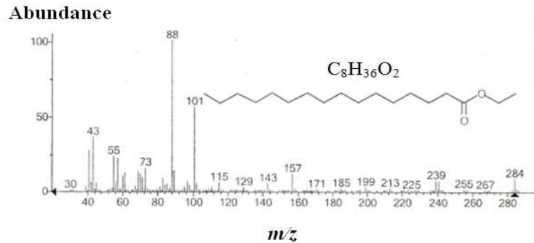
**Fig. 1: Mass spectrum of hexadecanoic acid, ethyl ester**
