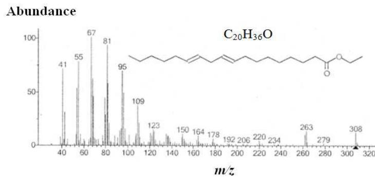
**Fig. 2: Mass spectrum of 9,12-octadecadienoic acid, ethyl ester**
