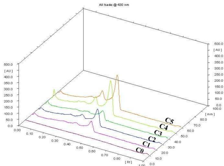
Fig. d: 3D densitogram of curcumin standard with the blank, Calibration curve was described by the regression equation,  $y = 40.899x + 470.22$  with  $R^2 = 0.9987$
