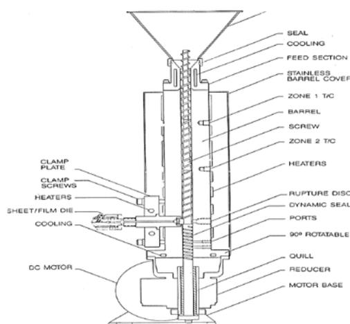
Fig. 1: Schematic diagram of the single screw extruder (Randcastle Extrusion Systems, Inc., USA).
