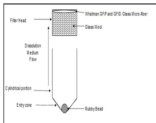
Fig. 2: Schematic diagram of the dissolution cell in the FTC apparatus.
