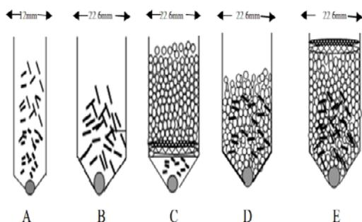
**Fig. 3: Schematic diagrams showing the five designs for IBU-HME pellets loaded into the FTC.**
