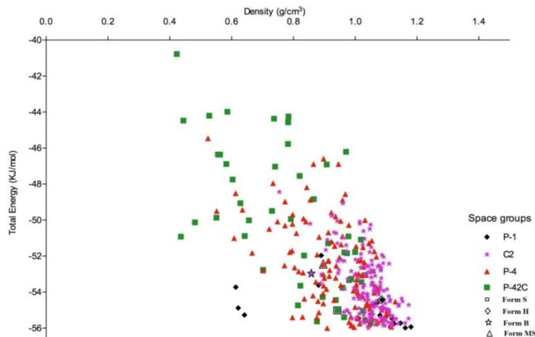
**Fig. 7: Crystal energy landscape within 16kJ/mol of global energy minimum. The lattice energy minima corresponding to the experimental crystal structure are also shown**
