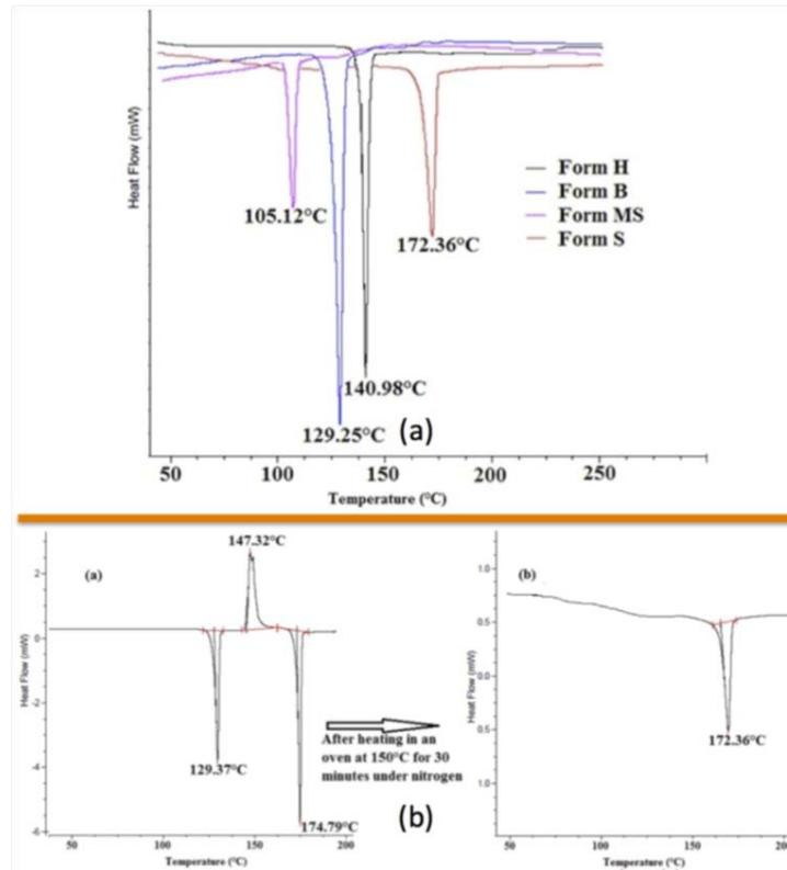
**Fig. 1: (a) DSC thermograms of nateglinide polymorphs, (b) DSC thermogram showing isolation of pure Form S**
