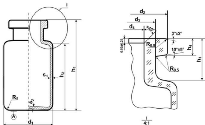
Fig. 1: Schematic view and dimensions of Injection Vials made of Neutral Borosilicate Glass Tubing according to the International Organization for standardization (ISO8362-1; 2009) [2].
