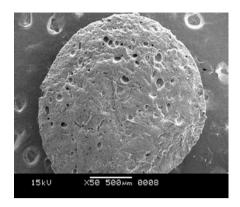
Fig. 4: SEM image of cross section of drug & oil incorporated alginate bead.
