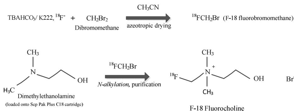
**Fig. 1: Synthesis of F-18 fluorocholine**
