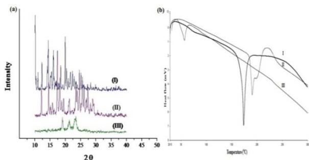
**Fig. 3:** (a) XRD analysis of (I) Native RAPA, (II) Native CUR, (III) (CUR+RAPA) loaded micelles, (b) DSC thermogram of (I) Native CUR, (II) Native RAPA, (III) (CUR+RAPA) loaded micelles.
