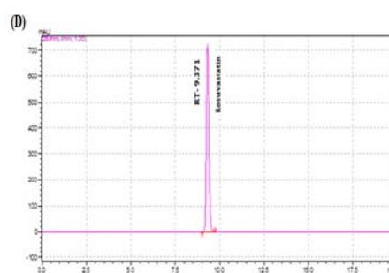
Fig. 5(D): Chromatogram of Standard solution of Rosuvastatin (50µg/ml).
