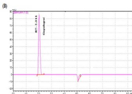
Fig. 5(B): Chromatogram of Standard solution of Clopidogrel (50µg/ml),
