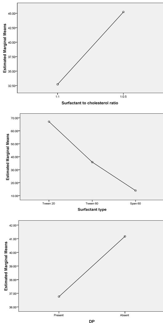
Fig. 8: Effect of surfactant type, surfactant to CH ratio and DP on the %Release efficiency
