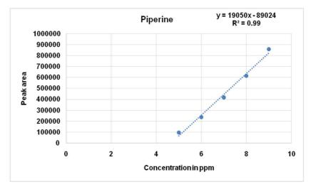
Fig. 7: Calibration curve of piperine
