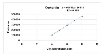
Fig. 6: Calibration curve of curcumin
