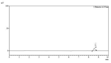
Fig. 4: Typical chromatogram of camphor standard solution
