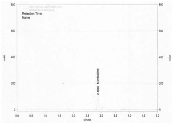
Fig. 7: Standard Chromatogram of Nimbolide 25 ppm/ml
