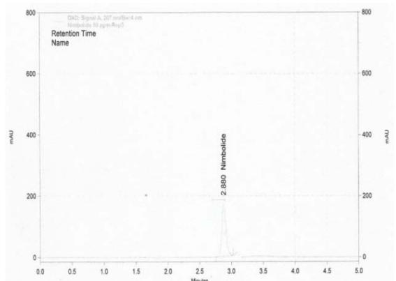
Fig. 8: Standard Chromatogram of Nimbolide 50 ppm/ml
