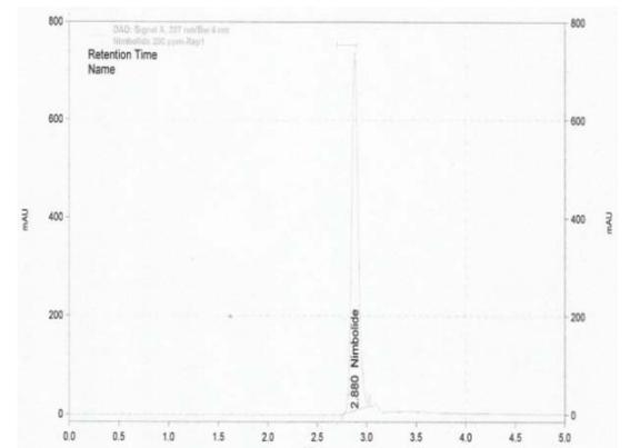
Fig. 10: Standard Chromatogram of Nimbolide 200 ppm/ml
