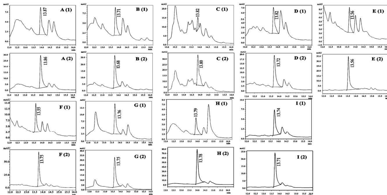
**Fig. 2: HPLC chromatograms of (1) herbal products (A-I), and (2) sildenafil citrate spiked in the herbal products (A-I)**
