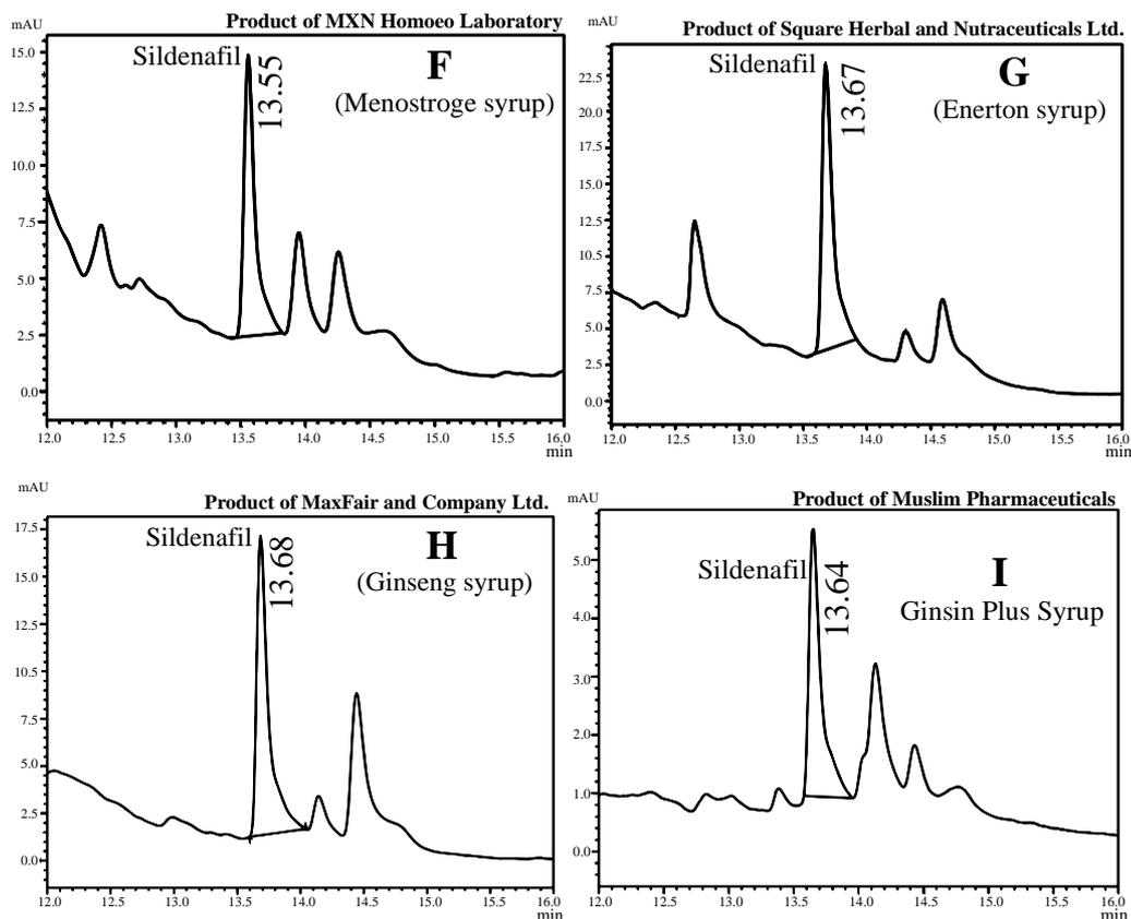
**Fig. 1: HPLC chromatograms of standard sildenafil citrate and herbal products (A-I)**
