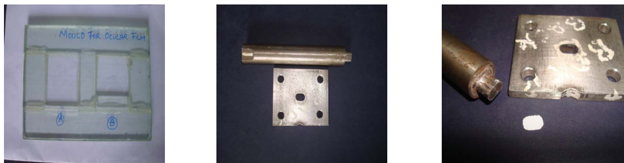
Fig. 2: In-House fabricated glass mould and punch die set and a ocular film of oval shape is shown in extreme right side.
