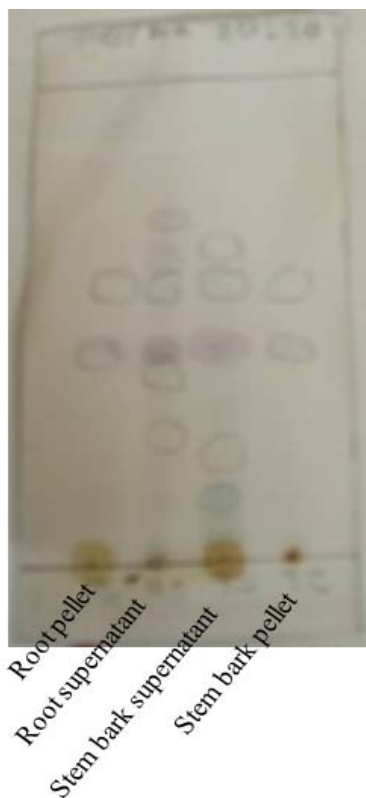
Fig. 1: Thin layer chromatography of different fractions of the whole hydroethanolic extract of roots and stem barks of Newbouldia laevis . Reading was realized invisible
