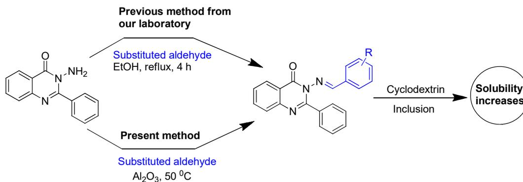
Fig. 2: Synthesis of substituted-3-(benzylideneamino)-2-phenylquinazolin-4(3H)-one using alumina as a catalyst
