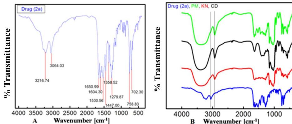
Fig. 7: IR spectrum of A) drug (2a) and B) drug (2a), cyclodextrin (CD), physical mixture (PM) and complex (KN), [blue line= drug; red line= complex; black line= CD; green line= PM]
