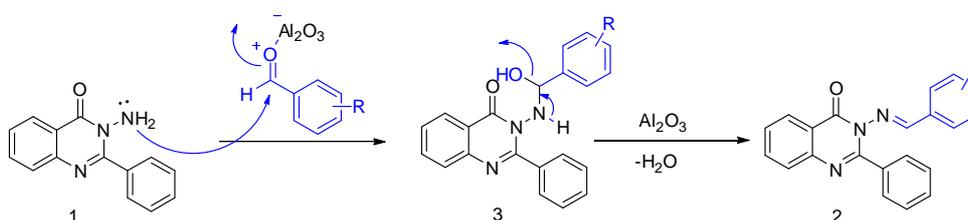
Fig. 4: Plausible mechanisms for solvent-free synthesis of substituted-3-(benzylideneamino)-2-phenylquinazolin-4(3H)-one using alumina
