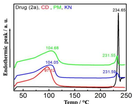
Fig. 8: DSC thermograms of drug (2a), cyclodextrin (CD), physical mixture (PM) and complex (KN). [mentioned with respective colour]
