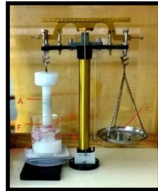
Fig. 1: Modified mucoadhesion test apparatus (Fabricated)
