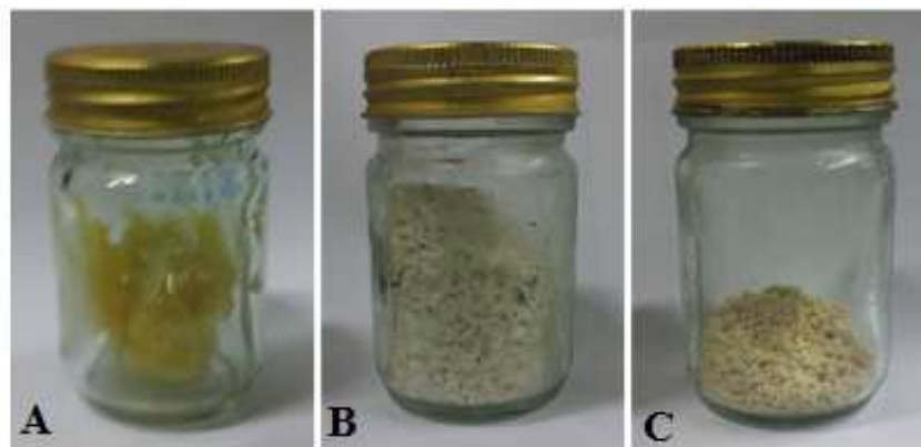
Fig. 2: The fresh pineapple juice powder from (A) freeze-dried process, (B) single- and (C) triple-layered pineapple juice granules
