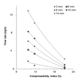
Fig. 4: Logarithmic relationship of compressibility indexes of GalenIQ 720, Helmcel 200 and metronidazole, against their flow rate, calculated by regression for orifices of different size.
