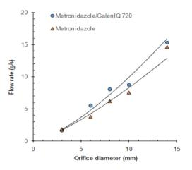
Fig. 10: Effect of the orifice diameter on the flow rate of metronidazole and its mixtures with GalenIQ 720.
