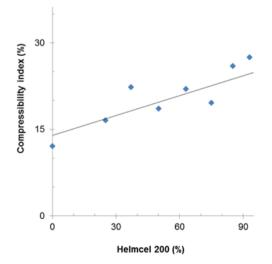
Fig. 11: Effect of the Helmcel 200 proportion on the compressibility index of its mixtures with metronidazole, expressed as the average obtained when using funnels with different size openings.
