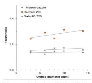
Fig. 2: Hausner ratio values obtained for GalenIQ 720, Helmcel 200 and Metronidazole, using funnels with orifices of different size.
