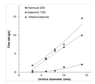
Fig. 3: Flow rate of powders of GalenIQ 720, Helmcel 200 and Metronidazole, when flowing through glass funnels with different size openings.
