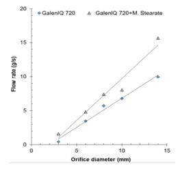
Fig. 7: Powder flow rate of pure GalenIQ 720 compared to the average of the flow rate of its mixtures containing up to 2% magnesium stearate when flowing through different size orifices.
