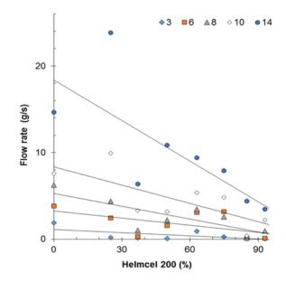
Fig. 12: Effect of the Helmcel 200 proportion on the powder flow rate of its mixtures with metronidazole, measured with funnels with different size openings (mm).
