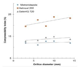
Fig. 1: Compressibility indexes (%) obtained for GalenIQ 720, Helmcel 200 and Metronidazole, using funnels with different opening sizes.
