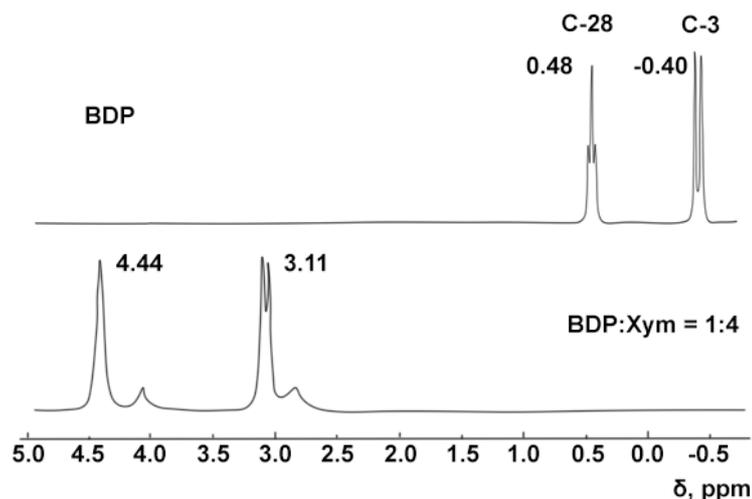
Fig. 6:  $^{31}\text{P}$ -NMR spectra of BDP (top) in  $\text{DMSO-d}_6$  and BDP-Xym mixture (bottom) in  $\text{D}_2\text{O}$ .  $\text{PPh}_3$  is a standard
