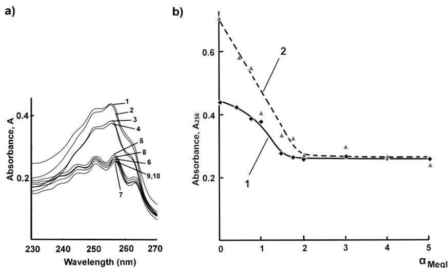
Fig. 7: The UV spectra in  $5.1 \cdot 10^{-4}\text{M}$  solutions of BDP in the presence of meglumine,  $C_{\text{LiClO}_4} = 1 \cdot 10^{-2}\text{M}$ : a)  $A = f(\lambda)$ ; b) the dependence of  $A_{256}$  absorption on the molar ratio of meglumine to BDP,  $A = f(\alpha_{\text{Megl}})$  in fresh solutions (1) and after 4 d (2),  $\alpha = n_{\text{Megl}}/n_{\text{BDP}}$
