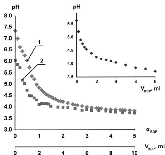
**Fig. 2: The pH dependence on molar fraction  $\alpha$ ,  $\text{pH} = f(\alpha_{\text{BDP}})$ ;  $\alpha = n_{\text{BDP}}/n_{\text{amine}}$ . The titration of 5.9·10<sup>-5</sup> M amine aqueous solution by 2.9·10<sup>-3</sup> M BDP ethanol solution: 1—meglumine; 2—xymedon. The inset shows  $\text{pH} = f(V_{\text{BDP}})$  after adding 2.9·10<sup>-3</sup> M BDP ethanol solution to water in a blank experiment. The initial amine solution volume was 100 ml**
