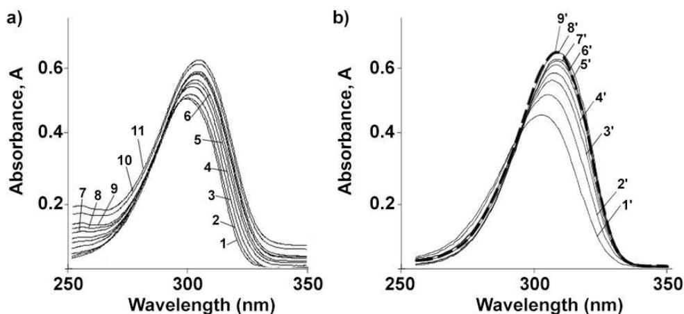
Fig. 4: UV absorption spectra of  $5.9 \cdot 10^{-5}$  M aqueous solution of xymedon and its protonated form obtained: a) in mixture with BDP;  $\text{C}_{\text{LiClO}_4} = 5.9 \cdot 10^{-4}$  M; b) in acetate-phosphate-borate buffer solution and in phytic acid (thick dashed line)
