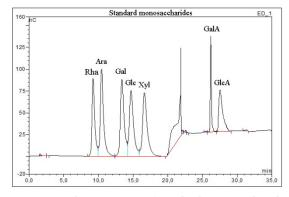
Fig. 2: HPAEC chromatogram of standard monosaccharides
