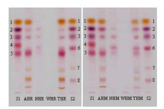
Fig. 1: TLC chromatograms of malvaceous polysaccharide; 1= rhamnose, 2=xylose, 3=arabinose, 4=mannose, 5=galactose, 6=glucose, 7=glucuronic acid, 8=galacturonic acid, S1=standard
