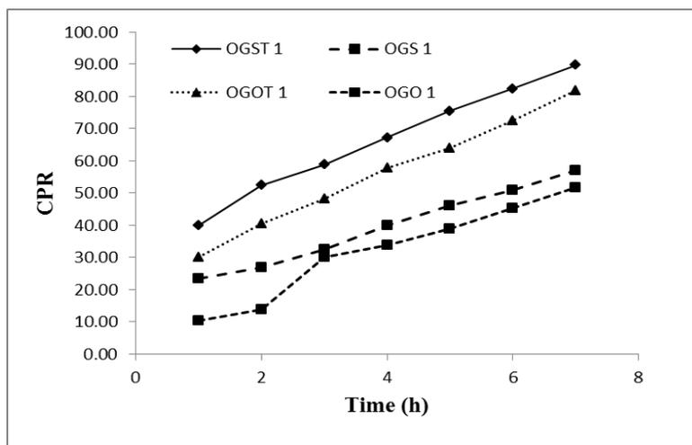
Fig. 3: CPR profile of soybean oil and olive oil-based oleogels at their CGCs. Error bars represent mean  $\pm$  standard deviation for 3 experiments (n=3)
