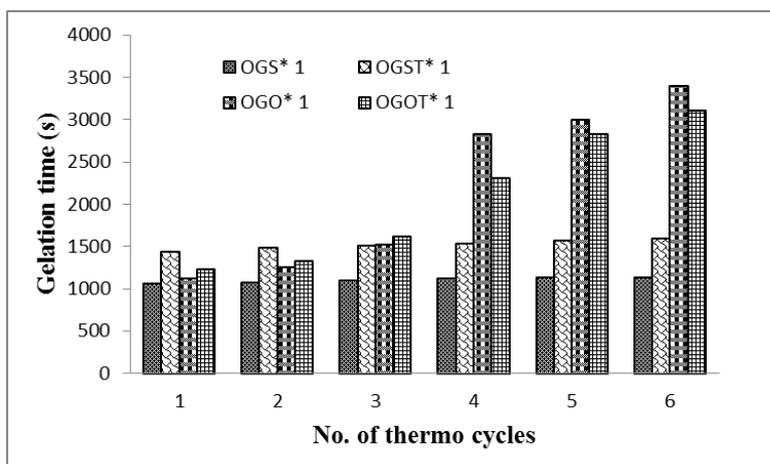
Fig. 4: Change in gelation time (s) with thermo cycles for oleogels of soybean oil and olive oil. Error bars represent mean  $\pm$  standard deviation for 3 experiments (n=3)
