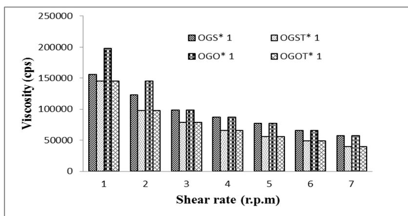
Fig. 2: Viscosity profile of soybean oil-and olive oil-based oleogels at their CGCs
