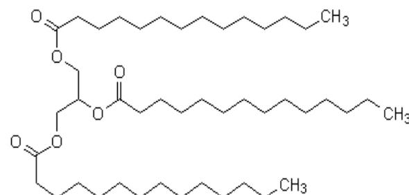
Fig. 3: Structure of Dynasan 114 have been myristic acid (C-14)
