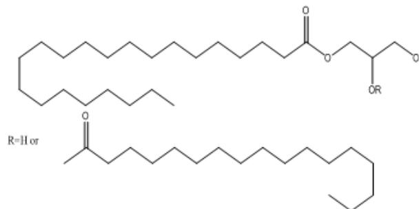
Fig. 1: Structure of Compritol ATO 888
