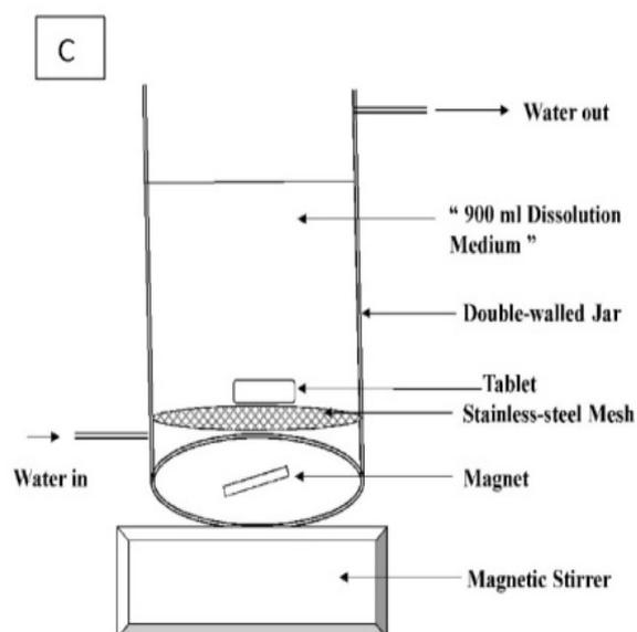
Fig. 1: Schematic diagrams of: (A) USP apparatus II, (B) USP apparatus IV, (C) Beaker method
