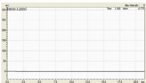
Fig. 3: Typical Chromatogram of Blank solution
