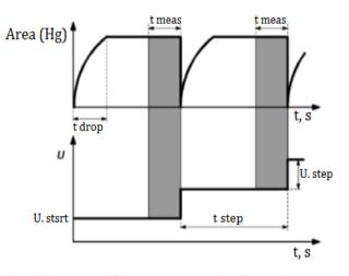
Fig. 1: The nature of the measurement using the static mercury drop electrode (SMDE)
