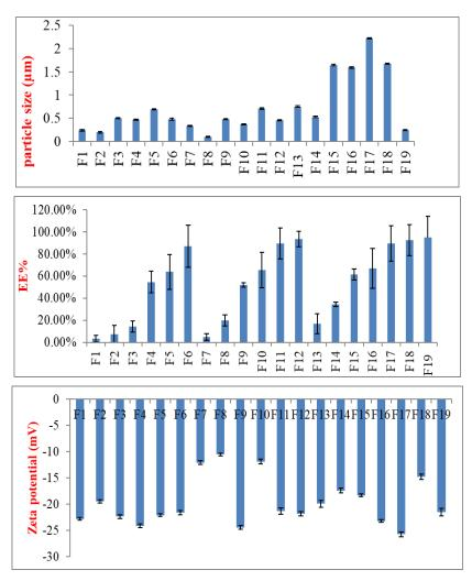
Fig. 3: Histogram of particle size, entrapment efficiency, and zeta potential of TFH loaded SLNs, (n= 3±SD)
