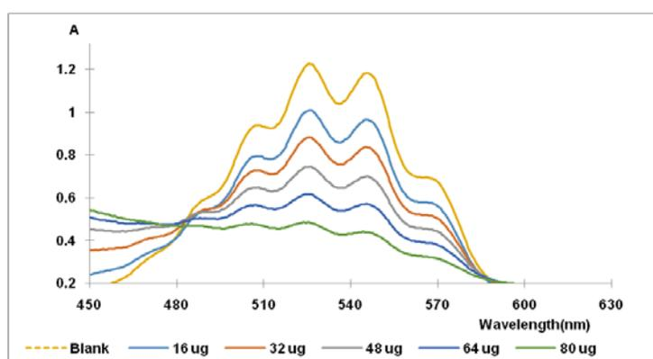
Fig. 2: Absorption spectrum of  $5 \times 10^{-4}$  mol/l KMnO<sub>4</sub>, 16-80 µg/ml of PIT with  $5 \times 10^{-4}$  mol/l KMnO<sub>4</sub>, at room T, for 30 min
