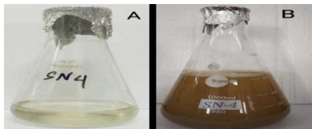
Fig. 1: Synthesis of silver nanoparticles from Strain NS-24: (A) Strain NS-24 supernatant before the addition of AgNO 3 , (Colorless), (B) Strain NS-24 supernatant after addition of AgNO 3 , (Brown)
