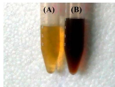
**Fig. 1: Digital images of diluted colloidal of AgNPs; (A) small particle size and (B) large particle size**
