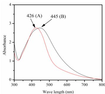
Fig. 2: UV-Vis absorption spectra of AgNPs; (A) small particle size, (B) large particle size
