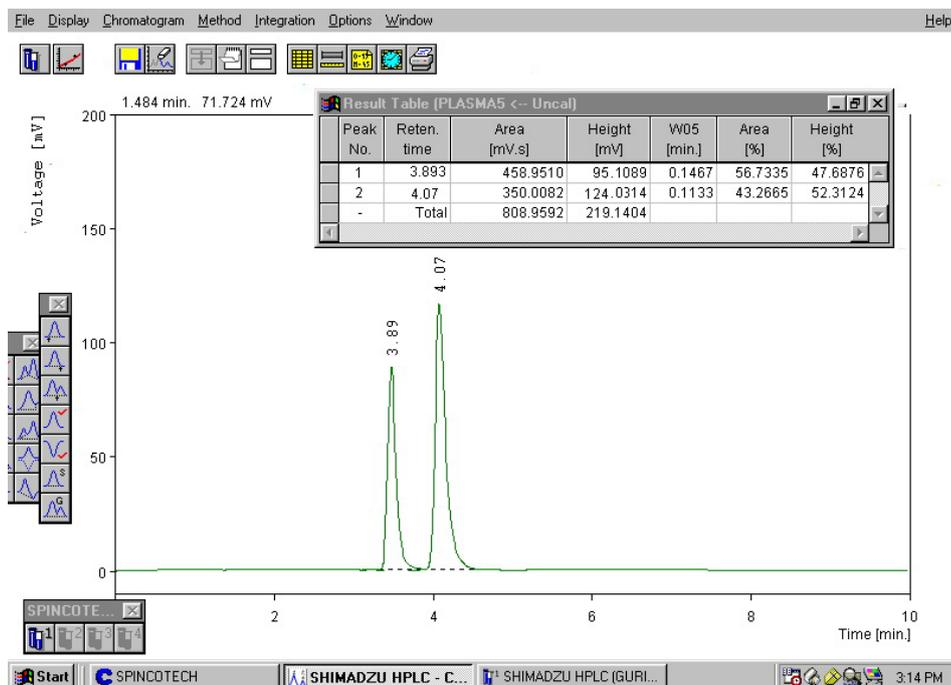
Fig. 3: Chromatogram for propranolol and metoprolol
