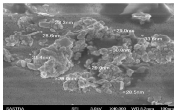
**Fig. 2: Scanning electron micrograph of copper oxide nanoparticles**
