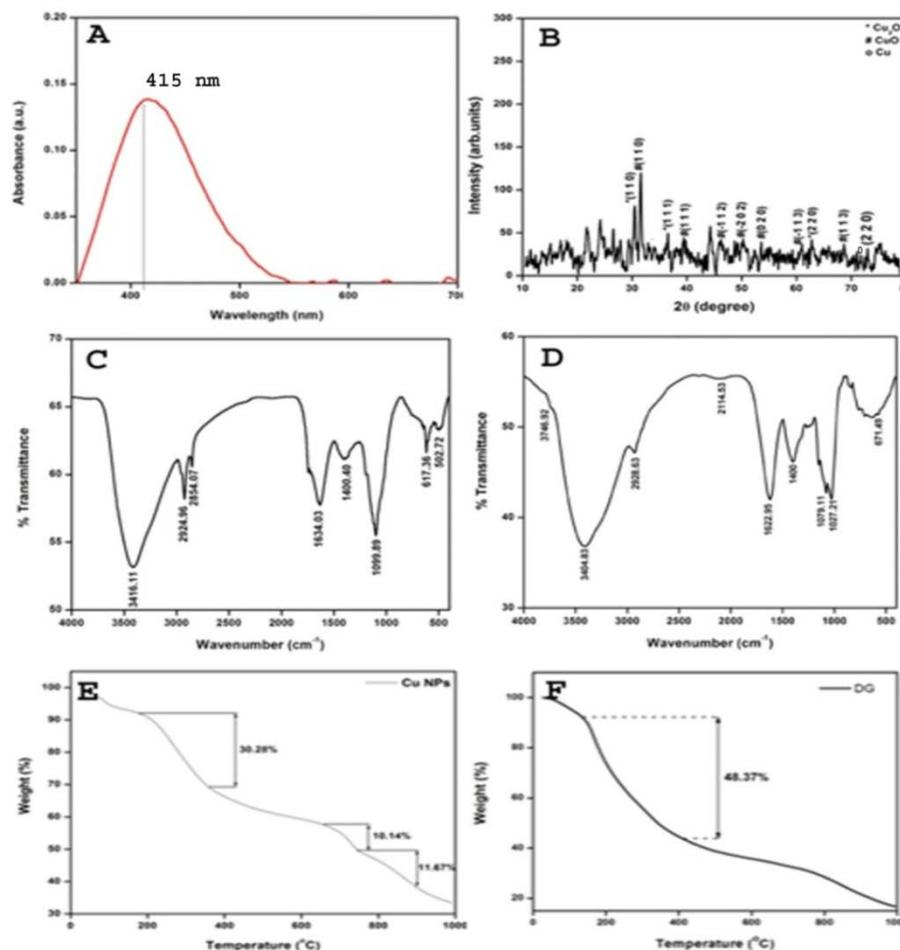
**Fig. 1: Characterization of copper oxide nanoparticle by UV-Visible spectrum, X-Ray Diffractometry and Fourier Transform Infrared Spectroscopy**
