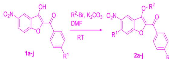
**Scheme 1: Synthesis of (3-alkoxy-5-nitrobenzofuran-2-yl)(phenyl)methanone derivatives (2a-j)**
