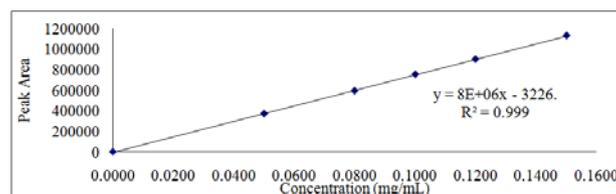
Fig. 8: Linearity curve for niacin
