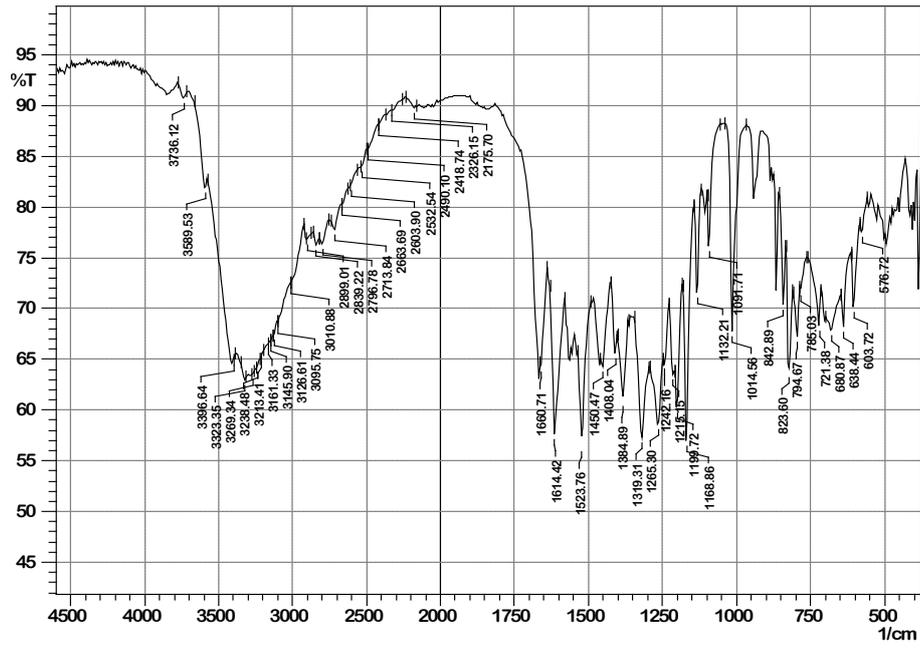
Fig. 2: FT-IR Spectrum of Quercetin
