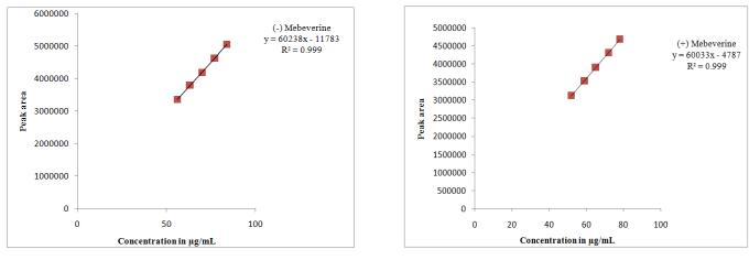
Fig. 6(a): Calibration curve of (-) Mebeverine
