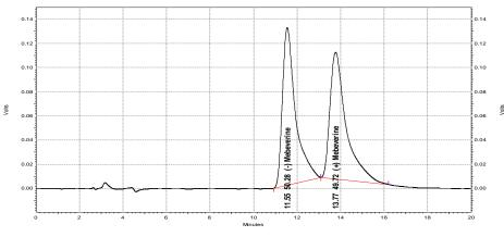
Fig. 3: Typical HPLC chromatogram of (-) Mebeverine and (+) Mebeverine
