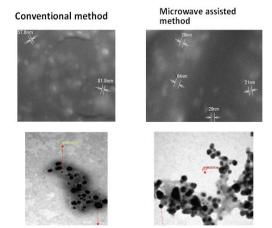
Fig. 3: SEM and TEM Micrographs of silver Nanoparticles of Brassica oleraceae
