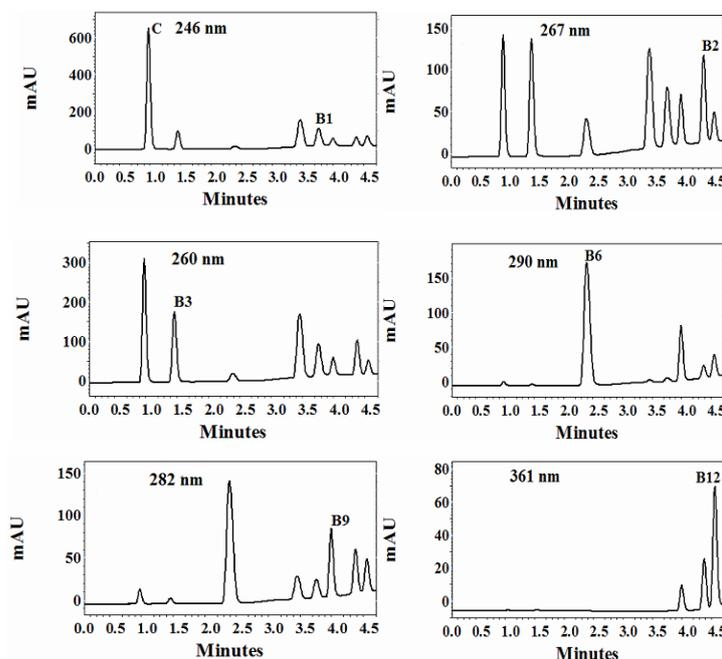
Fig. 2: Typical chromatograms of water soluble vitamins standard solution at 246 nm for C and B<sub>1</sub>, 267 nm for B<sub>2</sub>, 260 for B<sub>3</sub>, 290 for B<sub>6</sub>, 282 nm for B<sub>9</sub>, 361 nm for B<sub>12</sub> with methyl paraben as internal standard
