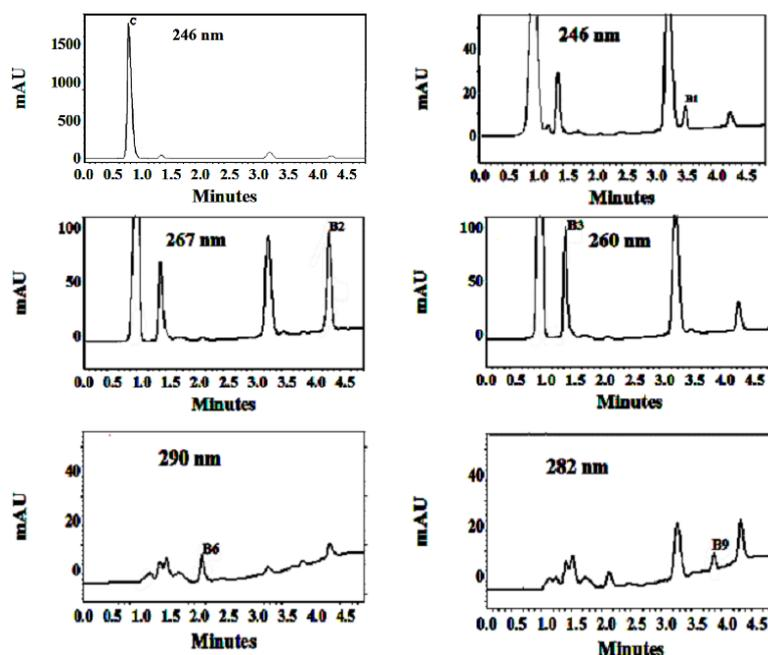
Fig. 4: Chromatograms of water soluble vitamins for (Nido) powder milk, with UV-DAD at 270 nm as a general view, 246 nm for C and B<sub>1</sub>, 267 nm for B<sub>2</sub>, 260 for B<sub>3</sub>, 290 for B<sub>6</sub>, 282 nm for B<sub>9</sub>, 361 nm for B<sub>12</sub> with methyl paraben as internal standard
