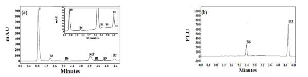
Fig. 3: (a): general view chromatogram of (B<sub>1</sub>, B<sub>2</sub>, B<sub>3</sub>, B<sub>6</sub>, B<sub>9</sub>, B<sub>12</sub> and C) and methyl paraben as internal standard for (Nido) powder milk, at 270 nm with UV-DAD. (b): Chromatograms of (B<sub>2</sub>, B<sub>6</sub>) for (Nido) powder milk, with FLD
