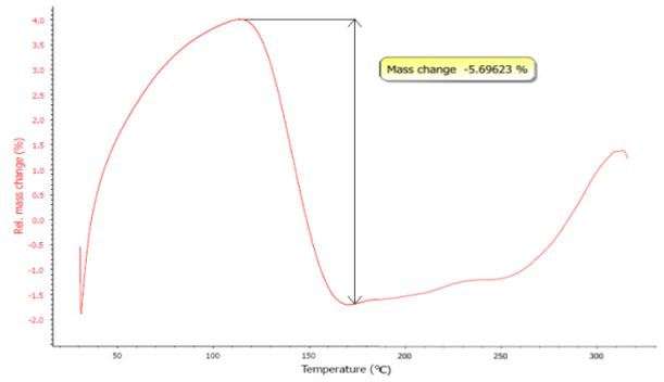
Fig. 19: TGA Thermogram of Sodium Sulfacetamide after Grinding for 180 min and Stored in 71% RH for 72 h
