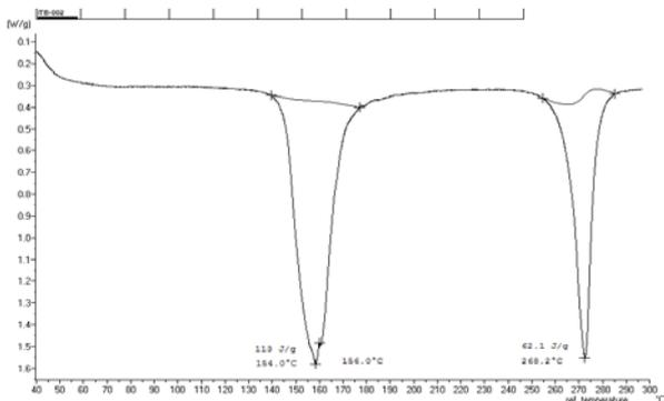
**Fig. 5: DTA Thermogram of sodium sulfacetamide**
