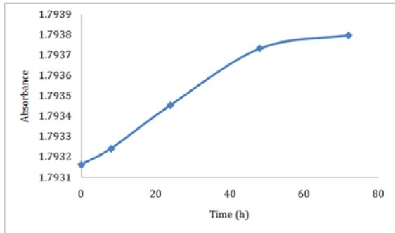
Fig. 16: IR Absorbance of Sodium Sulfacetamide versus Time of Storage in 99% RH
