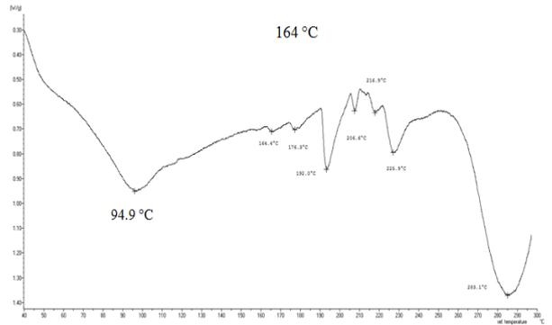
**Fig. 6: DTA Thermogram of neomycin sulphate**
