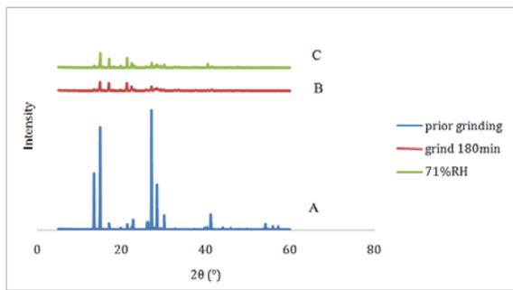
Fig. 17: PXRD Diffractogram of Sodium Sulfacetamide: prior Grinding (A), after Grinding for 180 min (B); Ground Sample for 180 min after stored at 71% RH for 72 h (C)
