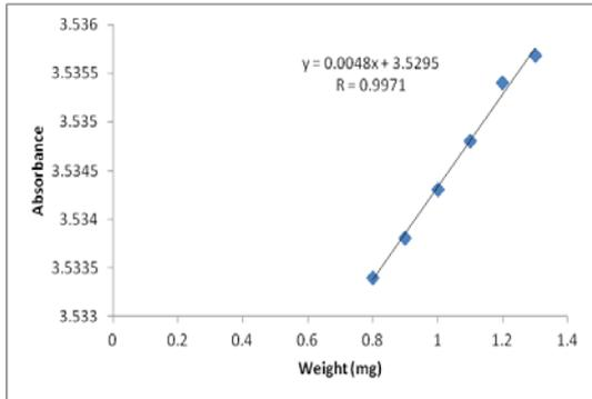
Fig. 9: FTIR Calibration graph of sodium sulfacetamide absorbance in different weights
