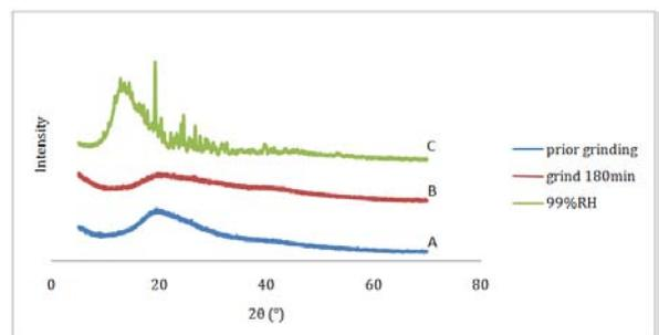
Fig. 22: PXRD Diffractogram of Neomycin Sulphate: prior Grinding (A), after Grinding 180 min (B), Ground Sample after Stored at 99% RH for 72 h (C)
