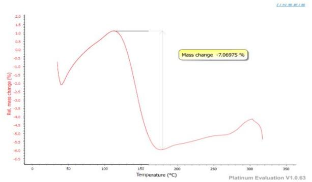
Fig. 12: TGA thermogram of sodium sulfacetamide after grinding for 180 min
