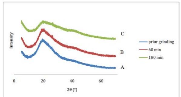
Fig. 13: PXRD Diffractogram of neomycin sulphate: prior grinding (A), after grinding for 60 min (B), and after Grinding for 180 min (C)
