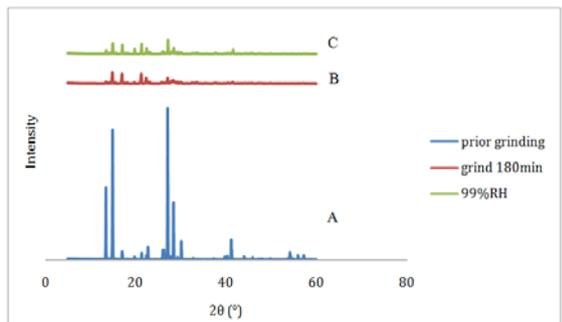
Fig. 18: PXRD Diffractogram of Sodium Sulfacetamide: prior Grinding (A), after Grinding for 180 min (B); Ground Sample for 180 min after Stored at 99% RH for 72 h (C)
