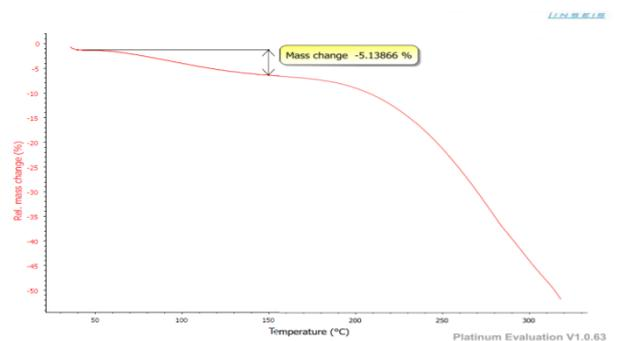
Fig. 14: TGA Thermogram of neomycin sulphate after grinding for 180 min
