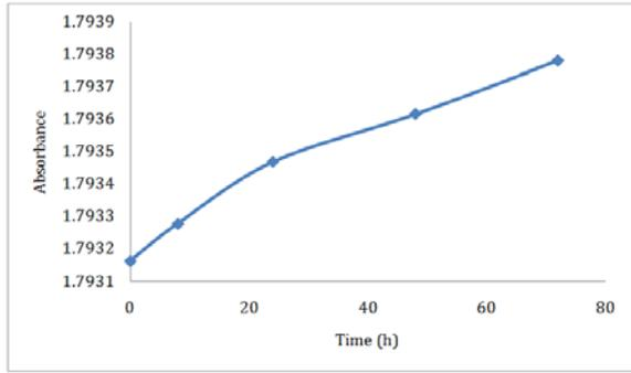
Fig. 15: IR Absorbance of Sodium Sulfacetamide versus Time of Storage in 71% RH
