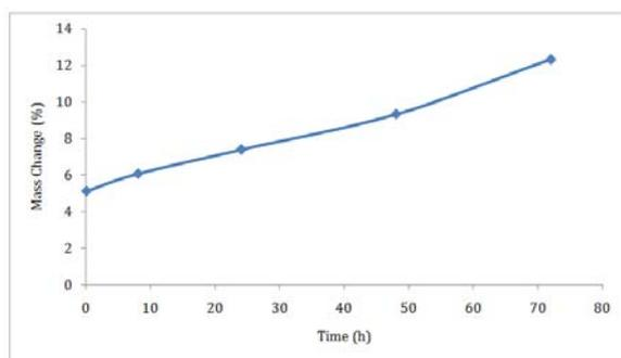
Fig. 24: Ground Neomycin Sulphate Hydration Curve after Storage in 99% RH for 72 h
