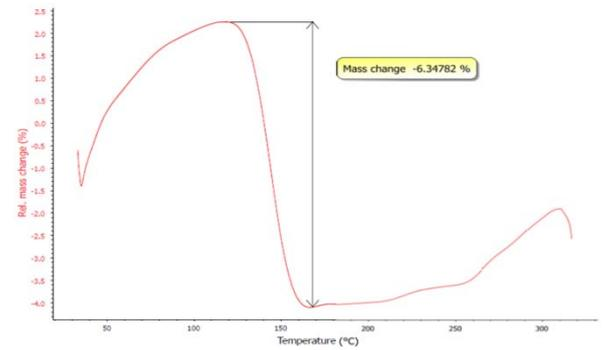
Fig. 20: TGA Thermogram of Sodium Sulfacetamide after Grinding for 180 min and Stored in 99% RH for 72 h
