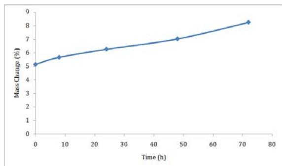
Fig. 23: Ground Neomycin Sulphate Hydration Curve, after Storage in 71% RH for 72 h
