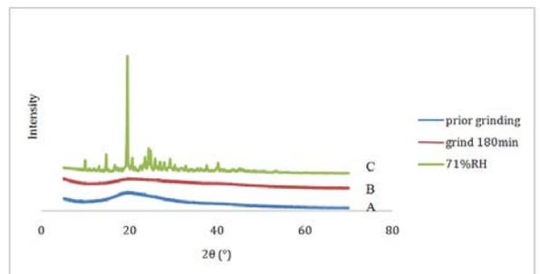
Fig. 21: PXRD Diffractogram of Neomycin Sulphate: prior Grinding (A), after Grinding 180 min (B); Ground Sample after Stored at 71% RH for 72 h (C)
