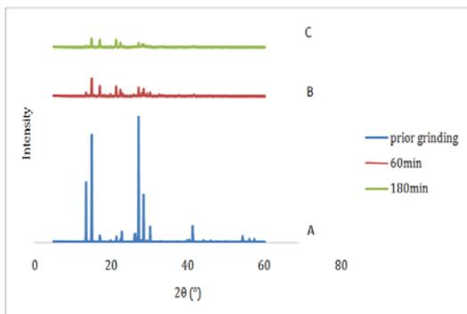
Fig. 11: Sodium sulfacetamide diffractograms: prior grinding (A), after grinding for 60 min (B), after grinding for 180 min (C)
