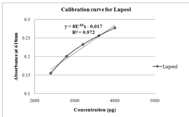
Fig. 1: It shows the calibration curve for lupeol standard from which Total Terpenoid Content of n-hexane extract of *M. ferrea* stamens was calculated
