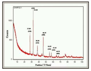
Fig. 4: X-ray diffraction analysis
