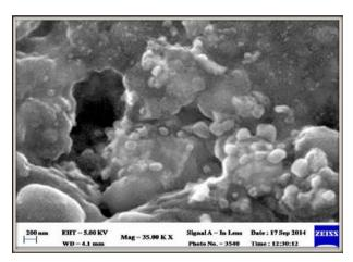
Fig. 3: Field emission-scanning electron microscopic image of AgNPs
