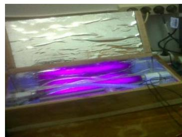
Fig. 4: A Photoelectrocatalytic reactor
