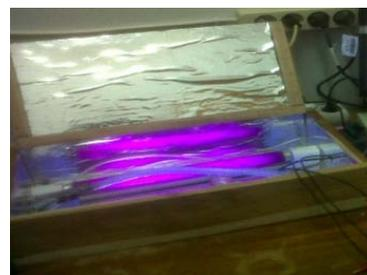
Fig. 4: A Photoelectrocatalytic reactor
