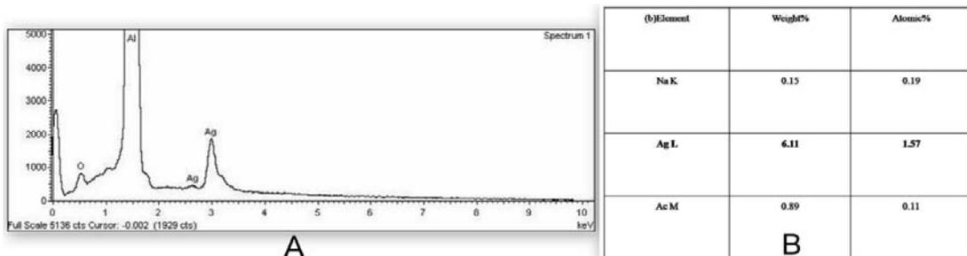
Fig. 6: EDAX of silver nanoparticles fabricated fabric, (A) shows the graph (B) shows the percentage of silver nanoparticles
