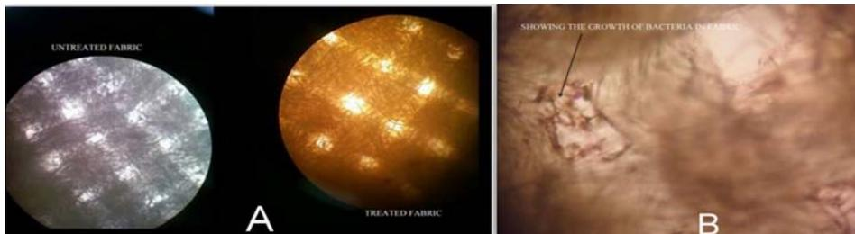
Fig. 4: Light microscope image of fabric. (A) silver nanoparticles fabricated into cotton fabric, (B) Silver nanoparticles untreated fabric- showing bacterial growth
