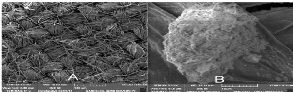
Fig. 5: SEM images of fabric. (A) Silver nanoparticles fabricated fabric, (B) Silver nanoparticles untreated fabric- showing the growth of bacteria
