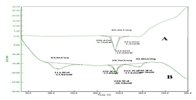
Fig. 4: DSC Thermogram of, (A): Nevirapine; (B): Best formulation F8
