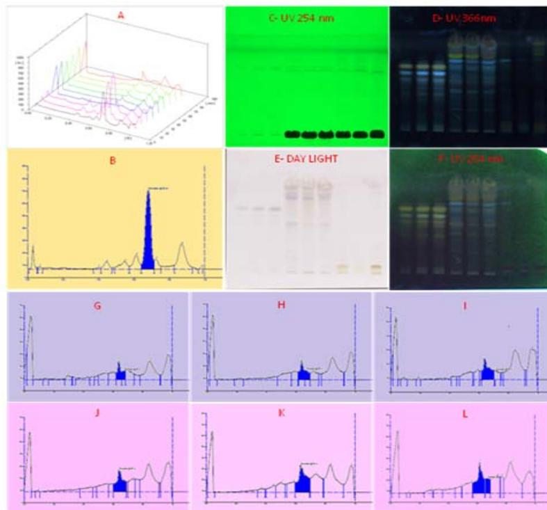
**Fig. 1: HPTLC fingerprint analysis on Cardiac Glycosides of *Thevetia peruviana* leaf extracts of three morphovariant plants using standard drug 'Peruvoside'**
