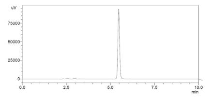
Fig. 2: Cephalexin reference standard solution Under proposed green chromatographic conditions
