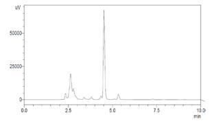
Fig. 7: Cephalexin solution under oxidative hydrolysis conditions
