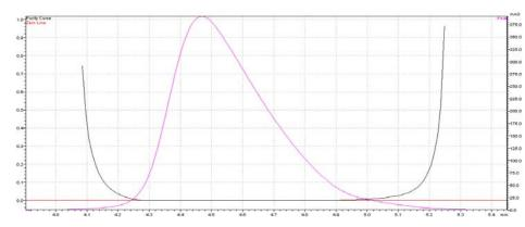
Fig. 4: Cephalexin peak purity by DDA detector, the purity factor was lower than the calculated threshold indicating the high selectivity of the proposed method
